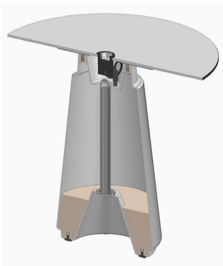
Electrified column with an inner tube made of steel with a diameter of 140 mm and bolted to the bottom of the column.
