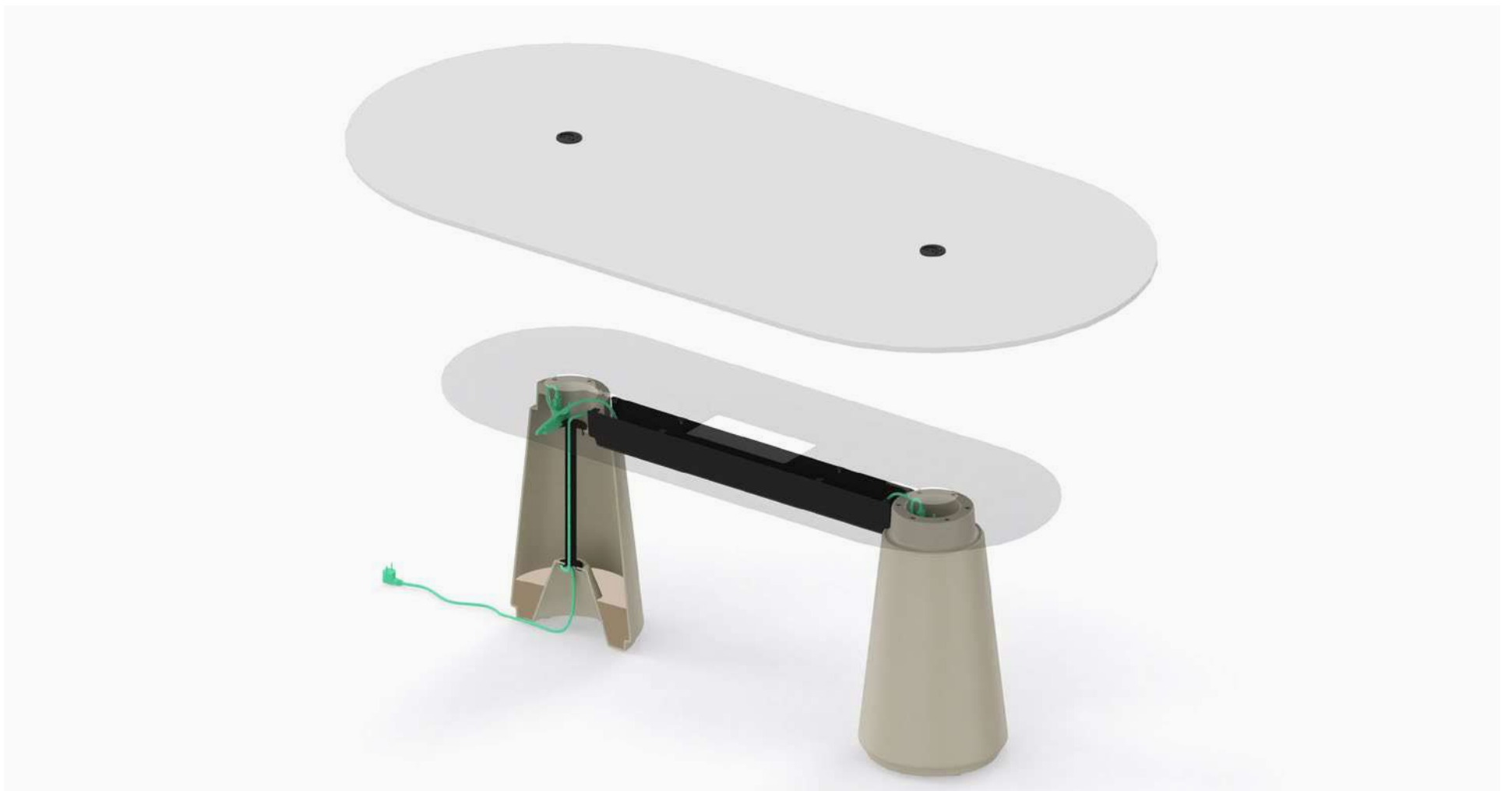
Integrated electrical management consisting of an electrified column and an electrification trunking connecting the two columns. One of the two columns is electrified with an inner tube made of steel with a diameter of 40 mm and bolted to the bottom of the column. The electrification tray is made of folded sheet steel with a thickness of 3 mm.
